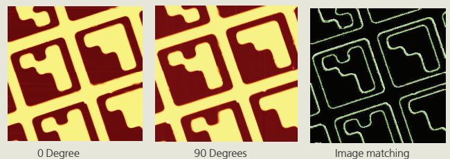
Figure 6. A good AFM should show no visible mismatch in the two orthogonal scans, demonstrating the excellent XY scan linearity.
